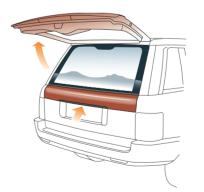
With all doors unlocked, press the switch on the bottom edge of the upper taildoor and lift to open.
